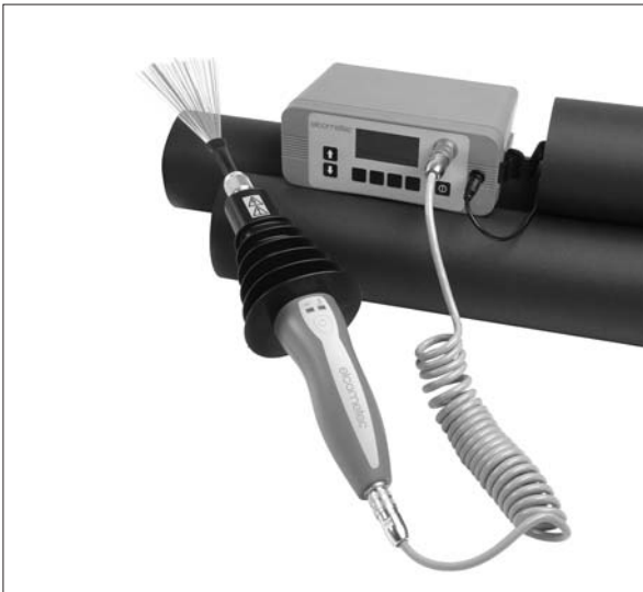
Image 8.2 Porosity probe for the tests under ISO 2746.
