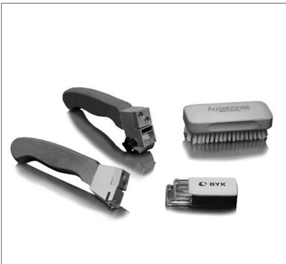
Image 8.4 Cross-cutting tool for determination of film adhesion under ISO 2409
